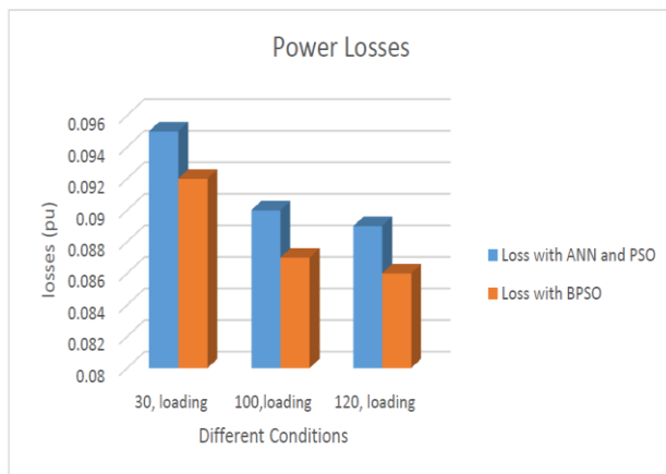
Fig. 7 Power Losses based on different generation at Talkha bus and loads at Damanhour 2 bus
